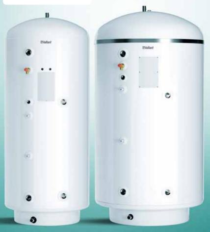
The new Vaillant cylinder range includes two large capacity cylinders and a complete range of accessories. The 500 and 800 litre uniSTOR's have impressive coil sizes, of 4.7m² and 7m² which are manufactured using high grade stainless steel, and pass the highest Vaillant standards and quality control requirements.
